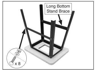
Figure 4. Long bottom stand braces attached.
